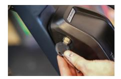
VOLITION uses a few battery cases which are all designed to "clip in" with a bit hand pushing. Please make sure the battery is in the "unlocked" otherwise it may not go in.
