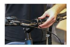
Install the handle bar with 4 screws (7 n.m)
