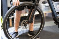
Once the front wheel is clipped in. Please push the bike down to pressure the wheel in a centred position and close the lever all the way in to lock it up securely.
