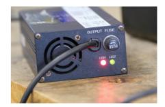
Chargers may appear slightly differently. LED (1) means the charger is getting the power from the wall.
